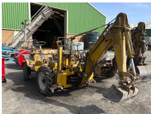
m420 THWAITES 2wd DUMPER/DIGGER Fitted with front stabiliser legs and Petter diesel engine
