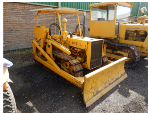
v358 BRISTOL PD48 diesel CRAWLER TRACTOR Serial No. 11326 Fitted with front dozer blade and canopy
