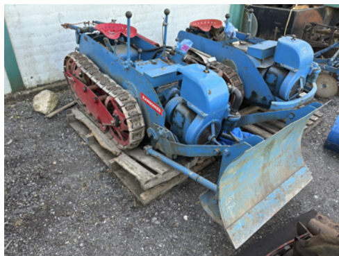
m400 RANSOMES MG6 petrol CRAWLER TRACTOR Serial No. 13126 Fitted with single cylinder petrol engine, front dozer blade, rear linkage
