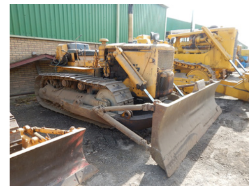
m361 CATERPILLAR D7 diesel CRAWLER TRACTOR Serial No. 17A16 51 Fitted with dozer blade, swinging drawbar and petrol donkey engine
