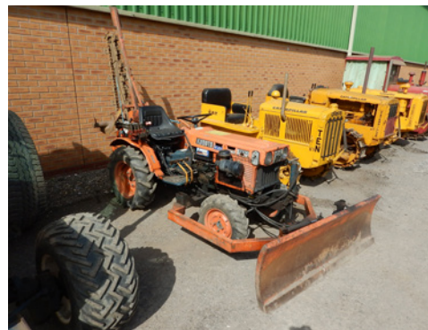
m301 KUBOTA B7100HST 4wd diesel COMPACT TRACTOR Serial No. 12349 Fitted with Kubota BK7A rear mounted trencher and hydraulic angle front blade. Showing just 983 hours
