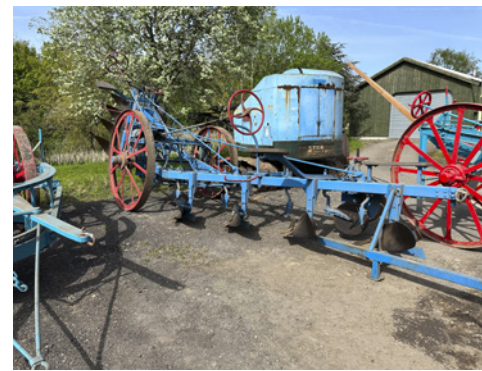
m380 Fowler anti-balance 4furrow steam plough with Ransomes UCN bodies, an earlier restoration
