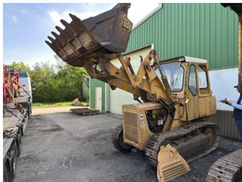
v419 INTERNATIONAL B100 series B diesel tracked LOADING SHOVEL Fitted with Drott 4in1 bucket Serial No. A020002B001253X
