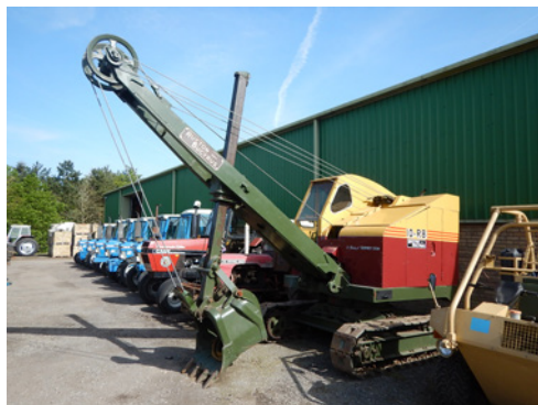
m356 RUSTON BUCYRUS 10-RB diesel DRAG LINE Serial No. R-B32358 Fitted with face shovel and Ruston & Hornsby engine. An earlier restoration
