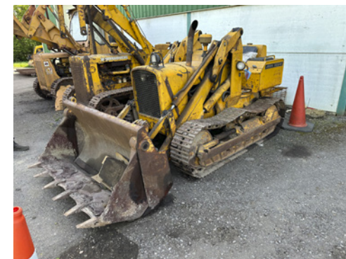
m417 JOHN DEERE 350 diesel tracked LOADING SHOVEL Fitted with Drott 4in1 loader bucket Serial No. 0008980D
