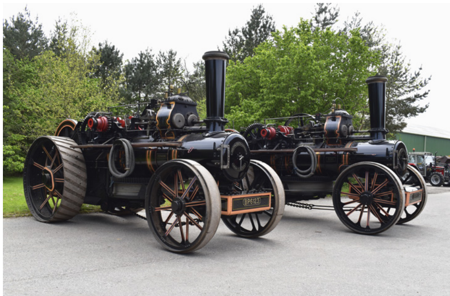
m376 1913 Fowler Ploughing Engines Class BB. Works Nos 13776 and 13777. Reg Nos. BP 6123 and BP 6121. 14 nhp. Double crank compound. 'Heroine' and 'Hero'.
