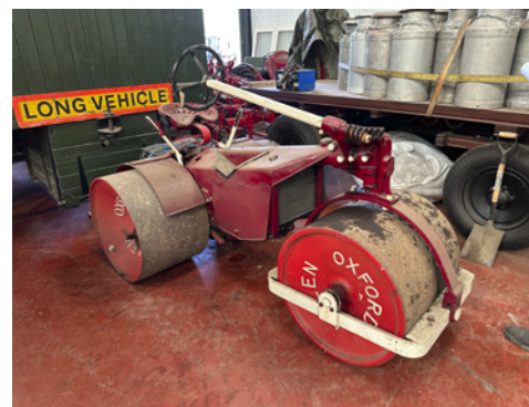
m285 ALLEN, Oxford RIDE-ON ROLLER Fitted with Austin 7 petrol engine
