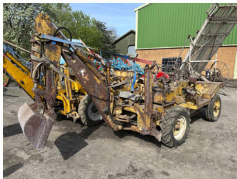
m421 THWAITES 2wd DUMPER/DIGGER Fitted with front stabiliser legs and Petter diesel engine
