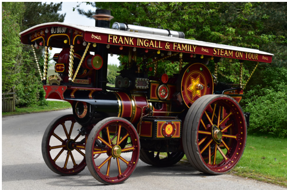
m378 1920 Garrett 4CD Showmans tractor. Works No. 33987. Reg no. BJ 5597. 4nhp. Double crank compound. Two speed. 'The Leader'
