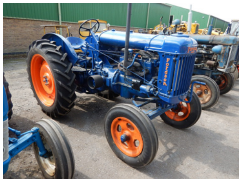
m326 FORDSON E27N petrol/paraffin TRACTOR Serial No. 1181314 Fitted with Type 7.7 high speed top gear, rear linkage and drawbar on good tyres all round
