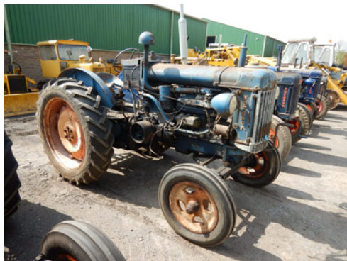
m325 FORDSON E27N 6cylinder diesel TRACTOR Reg. No. CJL 918 (expired) Serial No. 1127976 Fitted with a Perkins P6 engine, Type 7.7 high speed top gear, lights, rear linkage and drawbar on Goodyear diamond rear tyres. Purchased from a sale near Gedney, Spalding, Lincolnshire
