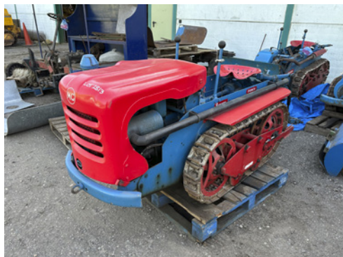
m399 RANSOMES MK40 diesel CRAWLER TRACTOR Serial No. 15243 Fitted with single cylinder Sachs diesel engine, electric start and rear linkage
