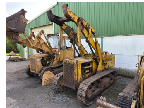
v418 INTERNATIONAL B100 diesel tracked LOADING SHOVEL Fitted with Drott 4in1 bucket Serial No. B8202
