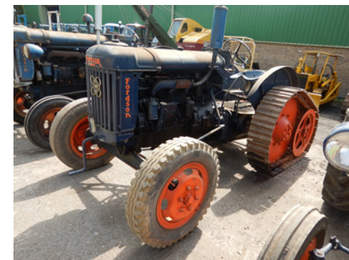
m324 FORDSON E27N DG4 6cylinder diesel TRACTOR Serial No. 1339 Fitted with a Roadless DG4 half-track conversion, Perkins P6 engine and side belt pulley
