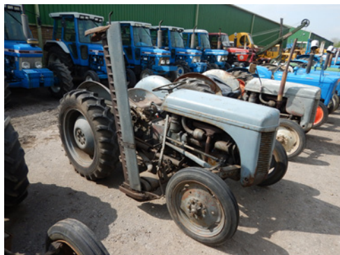
m336 FERGUSON TEF-20 diesel TRACTOR Serial No. TEF502492 Fitted with Ferguson mid-mounted finger bar mower and India Farm Tractor rear tyres
