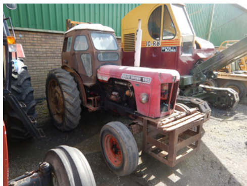
m355 DAVID BROWN 990 Implematic diesel TRACTOR Serial No. M990/AS/461632 Fitted with Sanderson 12/20 rear forklift and Sta-Dri cab. Supplied by Belton Bros & Drury Ltd, Langworth, Lincoln. A very original example
