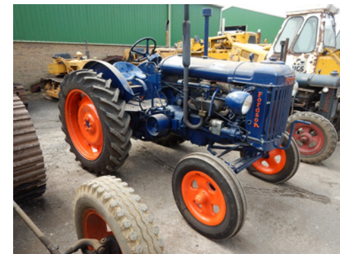
m323 FORDSON E27N petrol/paraffin TRACTOR Reg. No. CJR 852 (expired) Serial No. 1091517 An earlier restoration with electric start, drawbar, front lights on Goodyear tyres all round. Owned since 1970's
